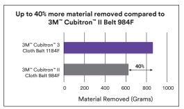
Results based on an automated, 10-minute grinding test on 304 stainless steel using 36" long belts. Total material removed: the total material removed in grams at 40 cycles.
