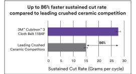
Results based on an automated, 10-minute grinding test on 304 stainless steel using 36" long belts. Error bars = 95% confidence interval. Cut rate: the total material removed in grams after 10 cycles minus total material removed in grams after 3 cycles divided by seven cycles. The unit is grams/cycles.
