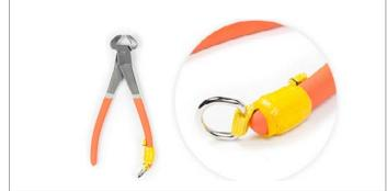
D-Rings plus Quick-Wrap Tape create an instant attachment point, with load ratings ranging from 2 lbs. (0.9 kg) up to 5 lbs. (2.3 kg) depending on model. Quick-Wrap Tape wraps around the D-Ring Attachment and conforms to the shape of the tool once it's stretched.
