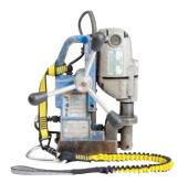
For heavier tools, consider using a Tool Cinch. Once applied, it creates a tether ready attachment point. Quick-Wrap Tape wraps around the stabilization wing of the Tool Cinch and conforms to the shape of the tool once it's stretched.
