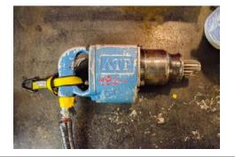
For heavier tools, consider using a Tool Cinch. Once applied, it creates a tether ready attachment point. Quick-Wrap Tape wraps around the stabilization wing of the Tool Cinch and conforms to the shape of the tool once it's stretched.
