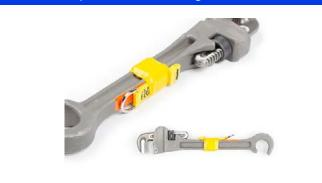
D-Rings plus Quick-Wrap Tape create an instant attachment point, with load ratings ranging from 2 lbs. (0.9 kg) up to 5 lbs. (2.3 kg) depending on model. Quick-Wrap Tape wraps around the D-Ring Attachment and conforms to the shape of the tool once it's stretched.
