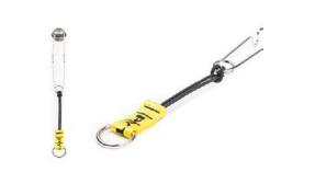
A D-Ring Cord creates a simple, secure and reusable attachment point for tools with pre-drilled holes or closed handles weighing up to 5 lbs. (2.3 kg).
