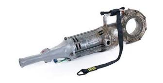
For heavier tools, consider using a Tool Cinch. Once applied, it creates a tether ready attachment point.
