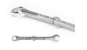
A Quick Ring can be fitted around a Combination Wrench as long as there is no risk of the ring slipping off either end of the tool (multiple Quick Ring sizes are available). This is an ideal attachment point for Combination Wrenches as it allows for the Quick Ring to rotate and move which helps prevent tangles, and stays out of the way of the user.
