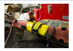
The Dual Wing Tool Cinch should only be used with a Bandsaw if the two stabilization wings do not interfere with the trigger of the tool. Because this is not always possible, the Single Wing Tool Cinch is strongly recommended in many cases as it will not interfere with the trigger of the tool.
