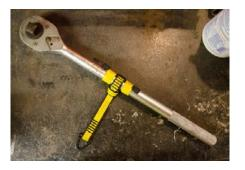
For heavier tools, consider using a Tool Cinch. Once applied, it creates a tether ready attachment point. Quick-Wrap Tape wraps around the stabilization wing of the Tool Cinch and conforms to the shape of the tool once it's stretched.
