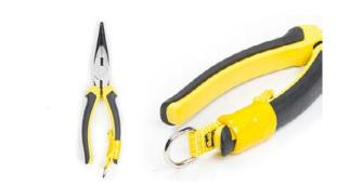
D-Rings plus Quick-Wrap Tape create an instant attachment point, with load ratings ranging from 2 lbs. (0.9 kg) up to 5 lbs. (2.3 kg) depending on model. Quick-Wrap Tape wraps around the D-Ring Attachment and conforms to the shape of the tool once it's stretched.
